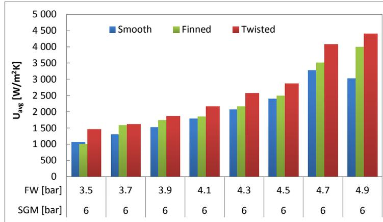
Figure 9: Average overall heat transfer coefficients
