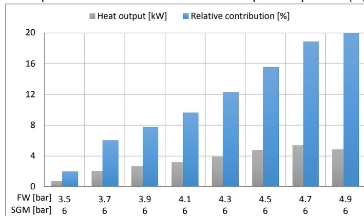
Figure 5: Heat output of the preheater and its contribution to the total heat output (10% CO<sub>2</sub>)
