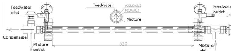
Figure 2: Single pass preheater with interchangeable middle section (installed in a vertical position)
