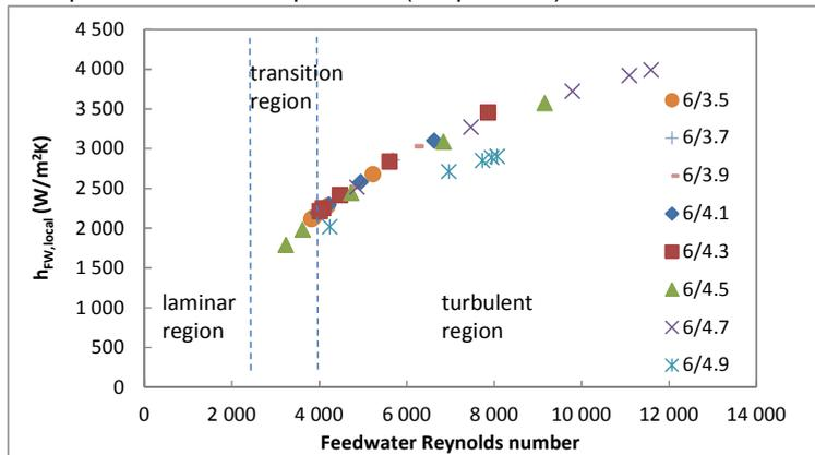
Figure 7: Heat transfer coefficients of feedwater in preheater (pressure in bar, mixture/feedwater)
