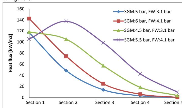
Figure 8: Heat fluxes in preheater (10 % CO<sub>2</sub> mass concentration at the DSG inlet)
