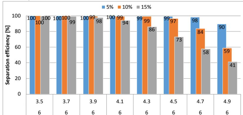
Figure 4: Effect of CO<sub>2</sub> presence in the mixture on the intensity of condensation (twisted tubes)
